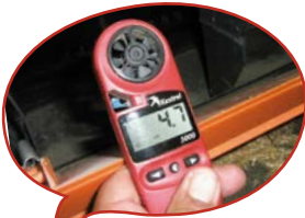
Measuring device The measurement of air velocity entering the barn through the supply air shows if the negative pressure of the the ventilation is correct .
